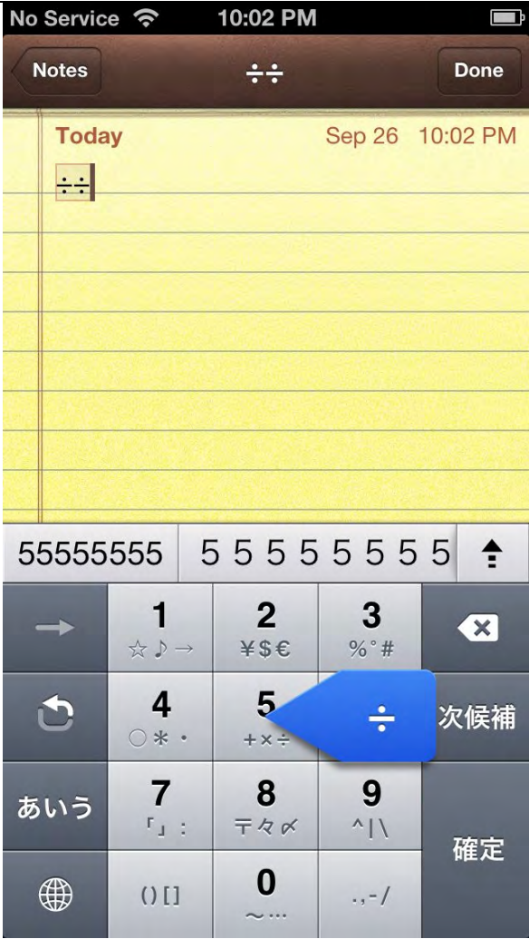
Sliding the finger in the up direction results in selecting and inputting the "x" key code:
