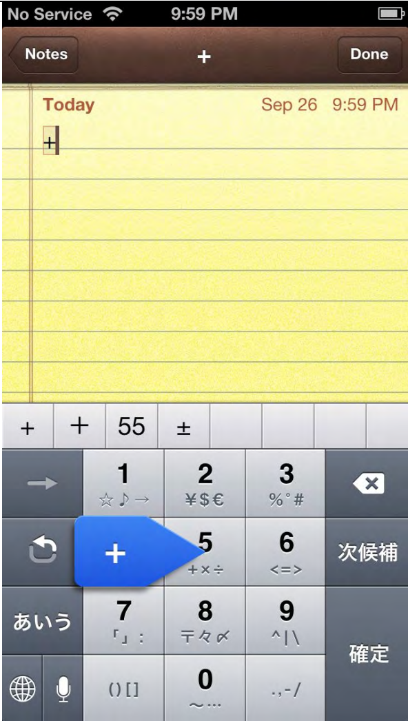
Sliding the finger to the right results in selecting and inputting the "÷" key code:
